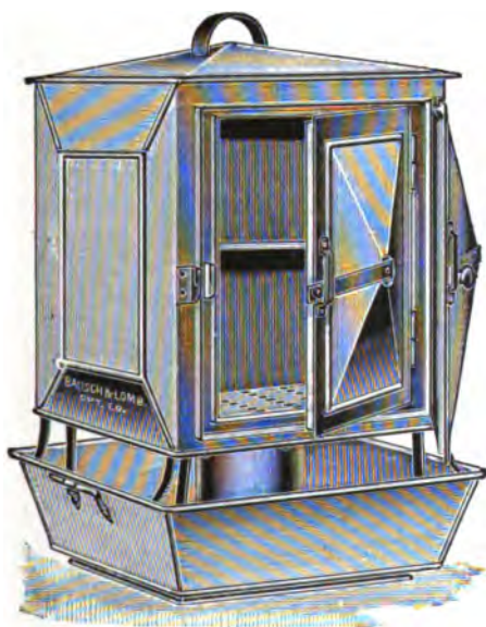
Fig. 39.—Arnold's steam sterilizer (Boston Board of Health form).
